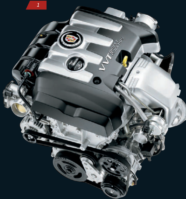
1 Producing 272 hp from just 2.0L of displacement, ATS's available Turbo powerplant is one of the most power-dense engines you can buy.
