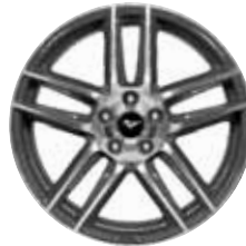
19" x 9" Front/19" x 10" Rear Sterling Gray-Painted Machined Aluminum Included: Boss 302 Laguna Seca Package
