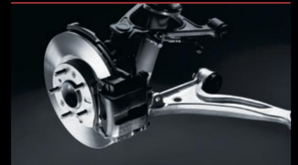
Every driver knows that when it comes to a sports car, slowing down is just as important as speeding up. The MX-5's ultra-responsive 4-wheel disc brakes with lightweight calipers come standard with anti-lock brakes and Electronic Brakeforce Distribution, ensuring linear fade-resistant stopping power whether you're on the track or on the road.
