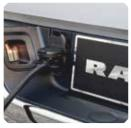
**THE CONNECTION.** Your trailer connector is easily accessible, with a separate adjacent lamp for easy connecting at night. All Ram 1500 models provide a 4- and 7-pin connector.
