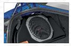
10-inch Powered Subwoofer. Provides powerful, deep bass and also assists in clean sound reproduction from all vehicle speakers. This is achieved by its integrated 100W amplifier and a passive crossover network. The self-contained unit mounts in the trunk. Manufactured for Subaru of America by Kicker.® Cannot be installed with Cargo Tray.
