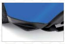
STI Rear Quarter Under Spoiler. Complete the look on the side of the BRZ with the addition of the rear quarter under spoilers. Kit includes both left and right rear guarter under spoilers.
