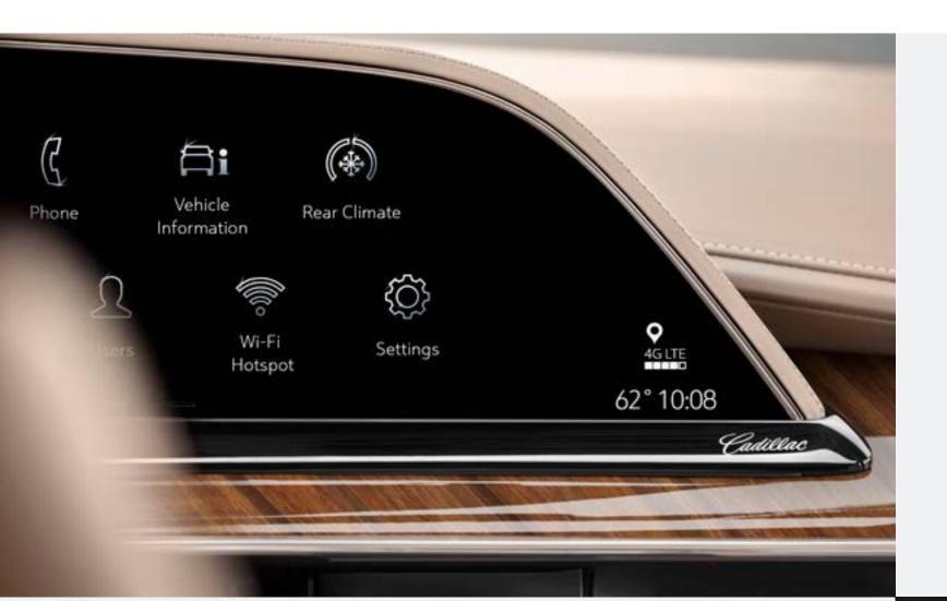
The OLED infotainment<sup>1</sup> and instrument panel works like your smartphone—a configurable interface with touch and swipe interaction.
