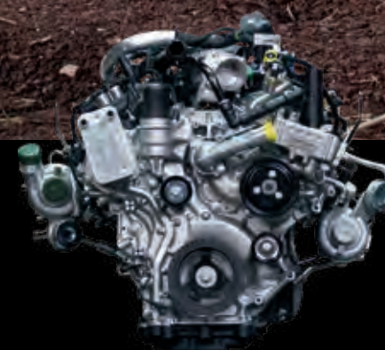
2.7L ECOBOOST 325 Max. HP 400 lb.-ft. Max. Torque
